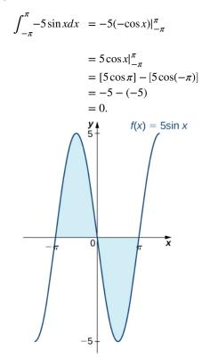
**Figure 1.36** The graph shows areas between a curve and the *x*-axis for an odd function.
