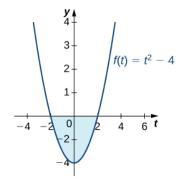
**Figure 1.28** The evaluation of a definite integral can produce a negative value, even though area is always positive.
