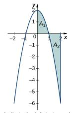
**Figure 1.18** In the limit, the definite integral equals area  $A_1$  less area  $A_2$ , or the net signed area.
