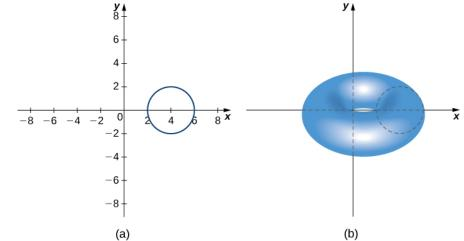
**Figure 2.74** Determining the volume of a torus by using the theorem of Pappus. (a) A circular region *R* in the plane; (b) the torus generated by revolving *R* about the *y*-axis.
